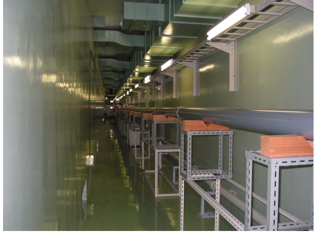
Fig. 4-1 Photos of a new laser beam line in the sub-tunnel of the test stand of the 50-MeV proton linac at KEK. The laser in the shielding box on the mounting stage (left one) and the shielding guided duct of 50 m in length viewed from the laser target side (right one).
