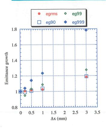
$\Delta X$ = deviation of SDTL rf center from Q-magnet center
