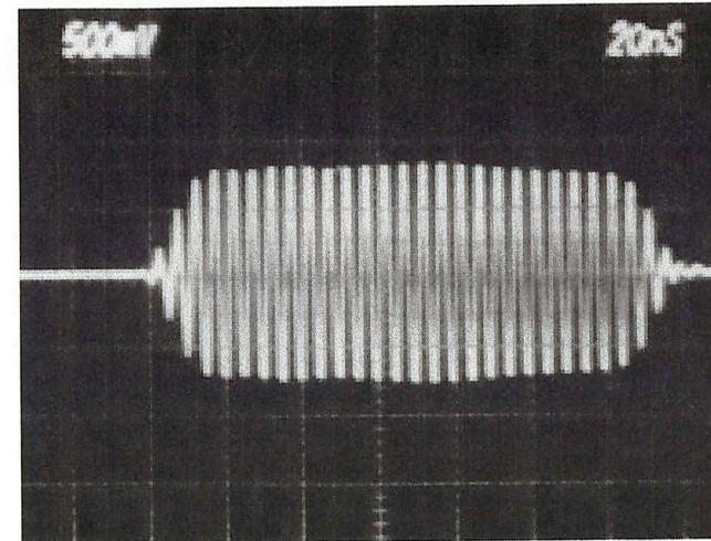
Calculated cavity field with an improved method. The initial amplitude ( $E_m$ ) of the incident power is 1.4 times higher. After some time,  $E_m$  is adjusted to 1. A rapid phase shift is added at a timing of turn-off. After some time (at about 33-th periods in this figure), the incident power is turned off.
