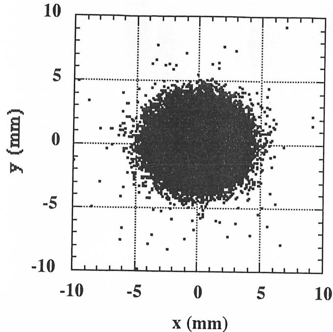
The output profile of the matched injection simulation. The number of particle is 48000.  $\alpha=0$ .
