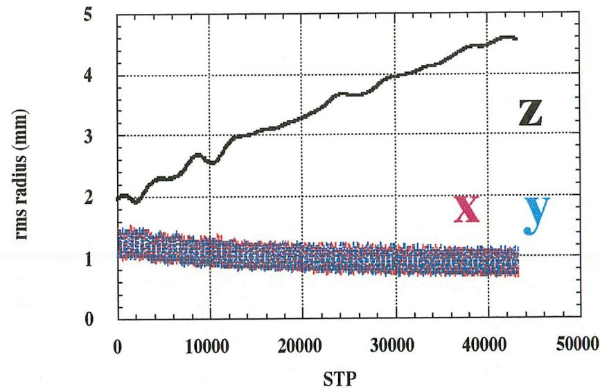
rms beam size vs. step number (energy)
