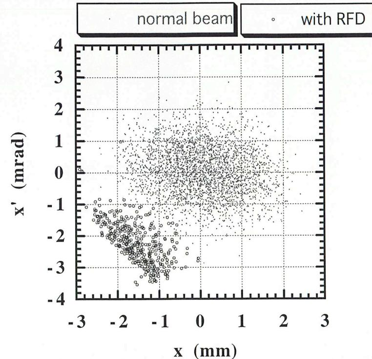
The transmission ratio for the micro bunch with a 10%-RFD field is more than 97%.
