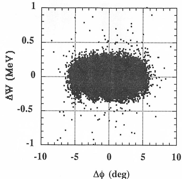
Longitudinal emittances after acceleration from 3 to 148 MeV. The left is results with the equipartitioning focusing method. The right is results with the constant phase advance method. The number of particles is 48000. The beam current is 30 mA.
