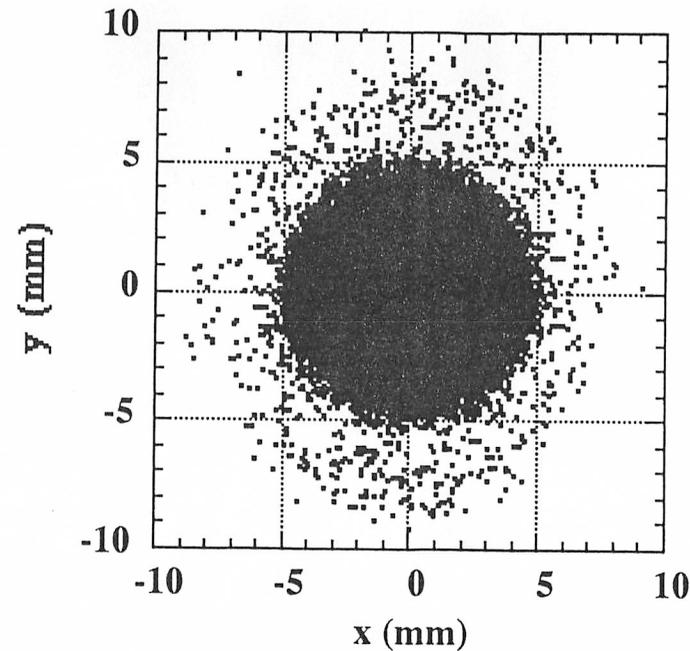
The output profile of the mismatched injection simulation. The number of particle is 48000.  $\alpha=0$ .
