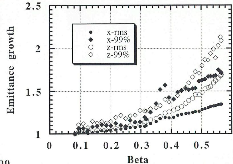
An rms beam size in the equipartitioning focusing method is connected smoothly from DTL to SDTL, although there is a transverse transition of length of focusing periods.
