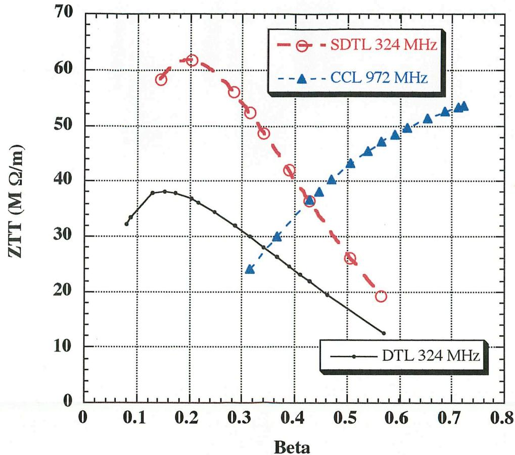
Effective shunt impedances used for the JHF proton linac.
