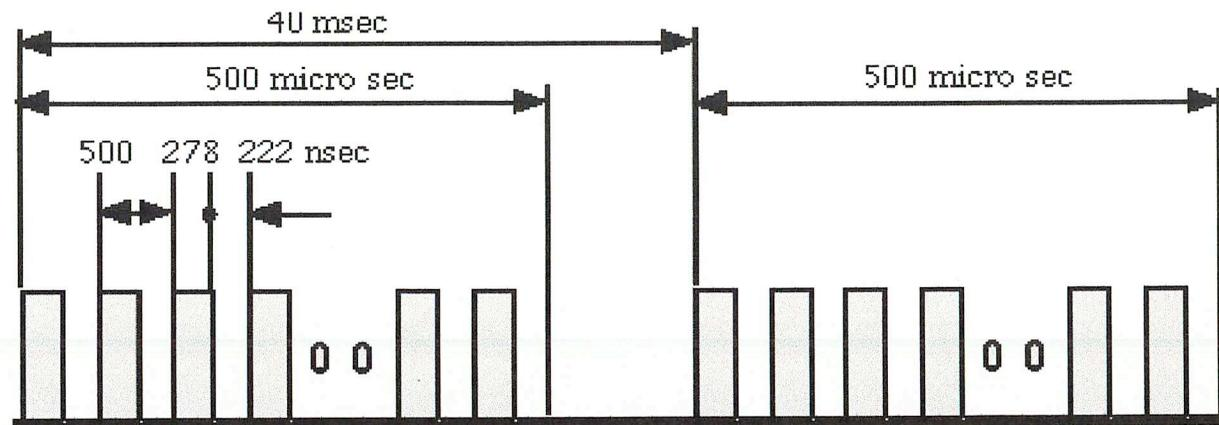
Required time structure of the bunch. A pulse length is  $500 \mu\text{sec}$ . A repetition rate is 25 Hz.
