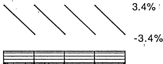
There is little change of acceptance and output energy width with this errors. Transmitted particles are 544 and energy width (90% full)=8.64 MeV.
