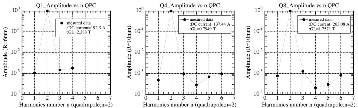
Fig. 3.1.2.3.14 Measured multipole components at the magnetic field center near the design current.
