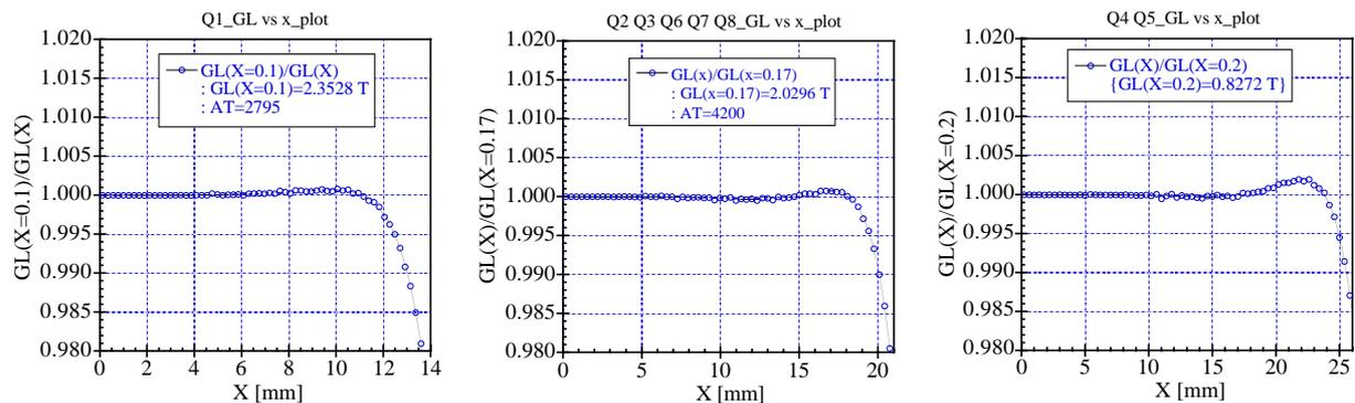
Fig. 3.1.2.3.13 Calculated radial distribution of the integrated field for all Q-magnets with the design current.
