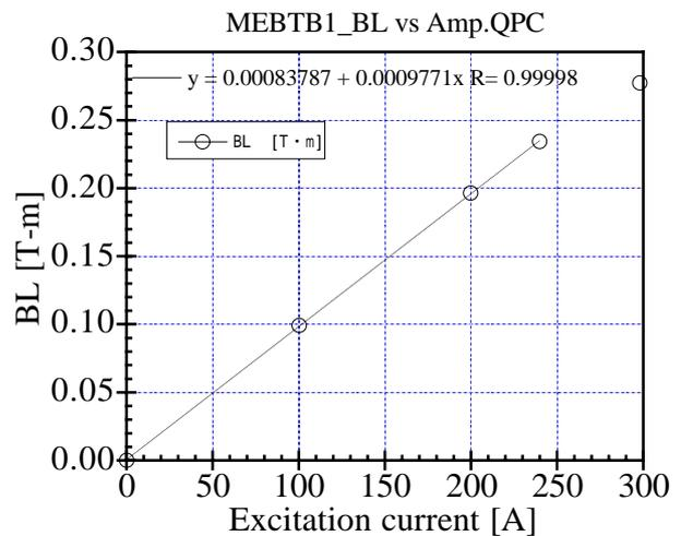
Fig. 3.1.2.3.16 Excitation curve of the bending magnet measured by a Hall probe.
