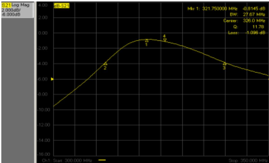
Fig. 3.1.2.3.5 Measured frequency spectrum of the single RFD.
