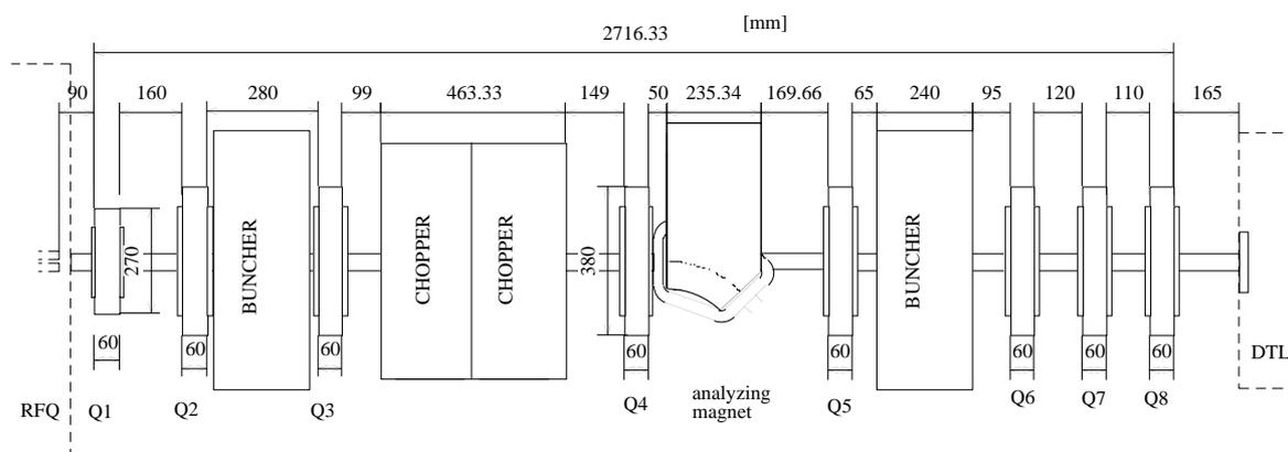
Fig. 3.1.2.3.10 Layout of the components in MEBT1.
