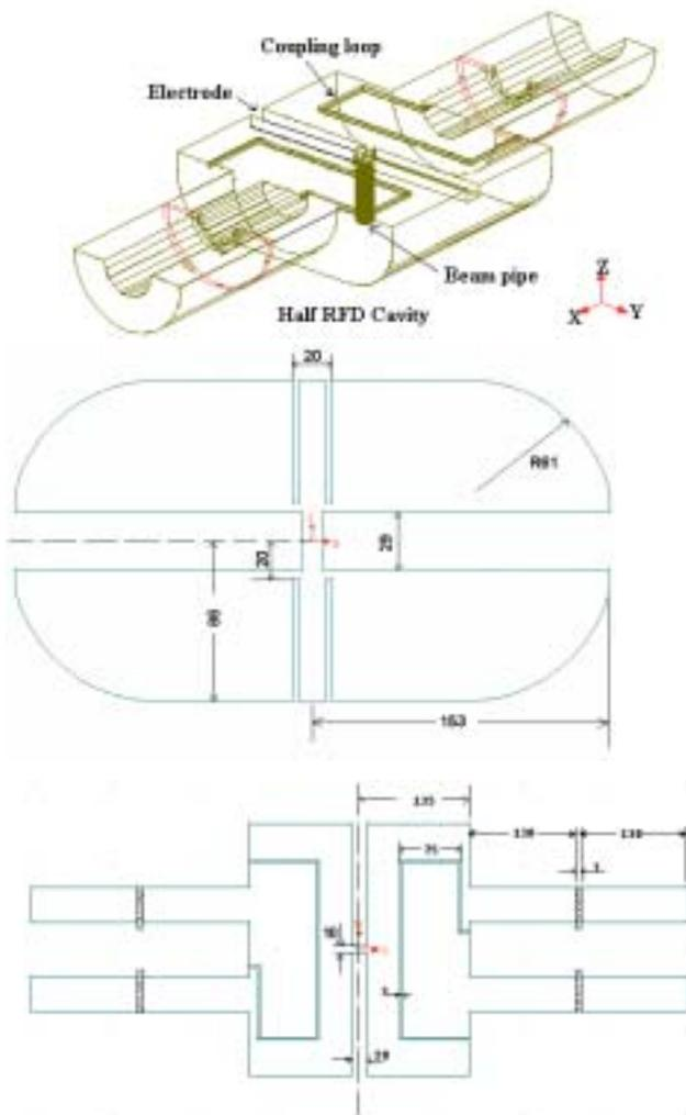
Fig. 3.1.2.3.3 Geometry of the RFD.
