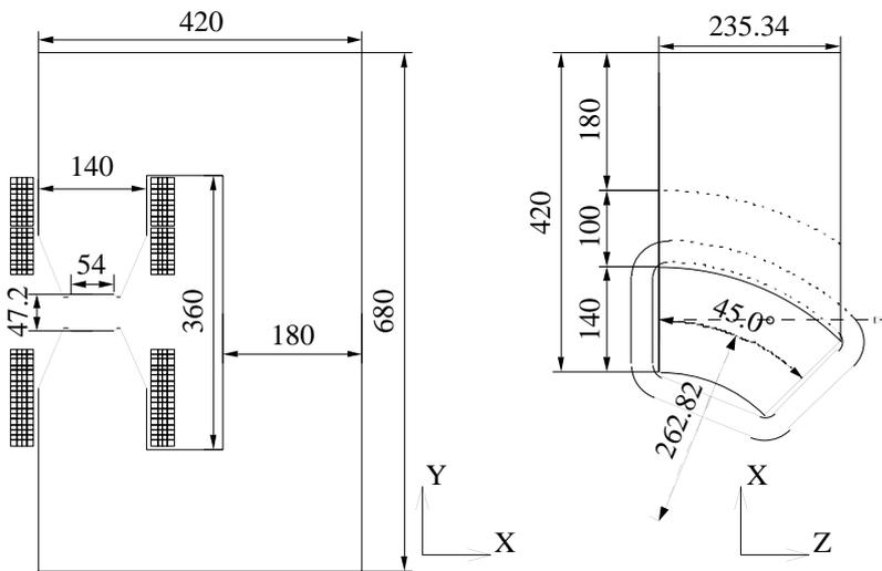
Fig. 3.1.2.3.12 Cross-sectional view of the energy analyzing magnet.
