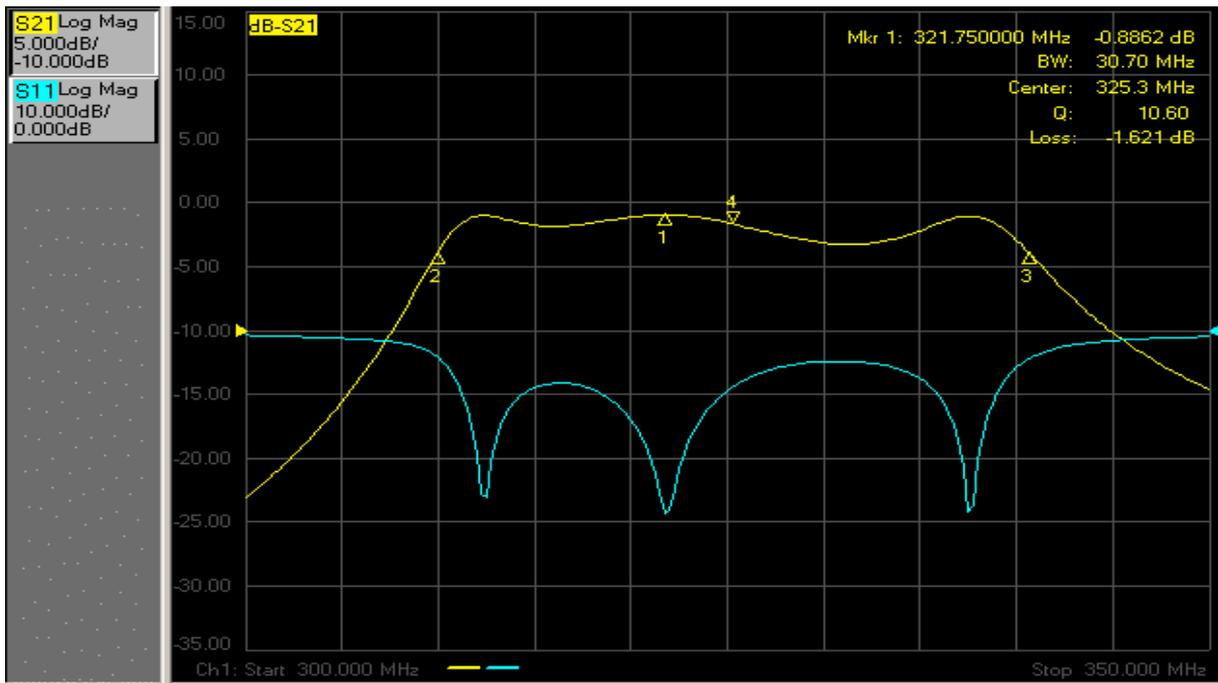
Figure 3.1.2.3.7 Measured frequency spectrum of the coupled RFD system.
