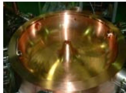
Fig. 3.1.2.3.2 A half part of the buncher cavity before brazing.
