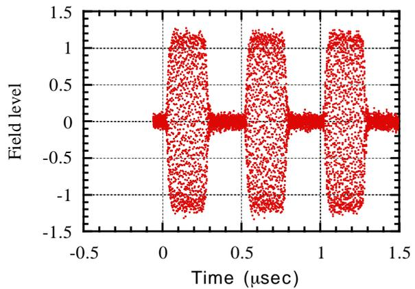
Fig. 3.1.2.3.6 RF field amplitude in the single RFD with a 30 kW input power.
