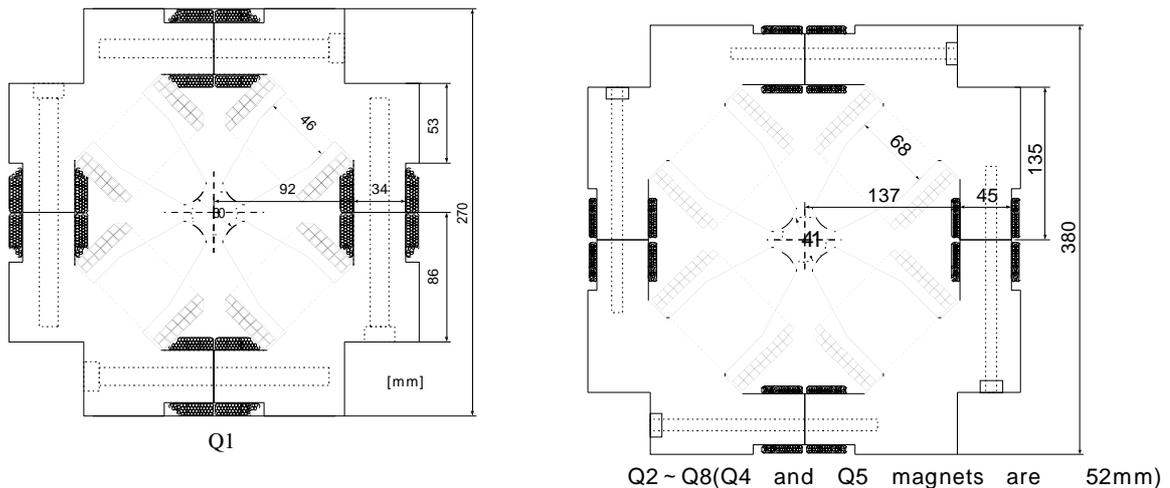
Fig. 3.1.2.3.11 Cross-sectional view of the quadrupole magnets.
