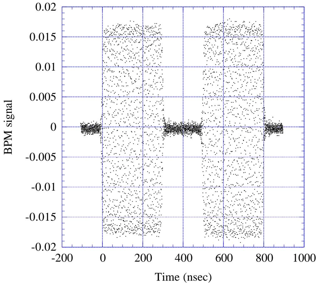
Figure 3.1.2.3.17 Measured signal of a chopped beam pulse from one of the electrode of the beam position monitor installed into Q8 (the last quadrupole magnet in the MEBT).
