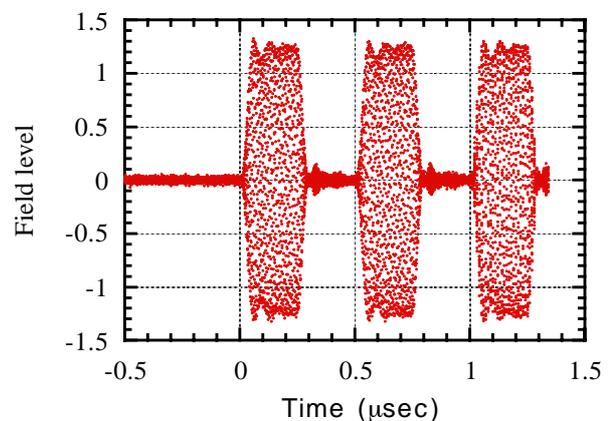
Fig. 3.1.2.3.9 RF field amplitude in the second cavity of the coupled RFD with a 30-kW input power.
