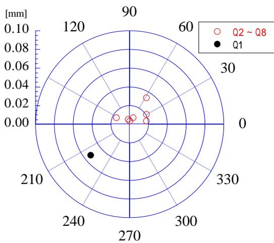
Fig. 3.1.2.3.15 Measured deviation of the magnetic field center from the mechanical one near the design current.
