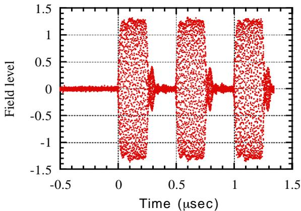
Fig. 3.1.2.3.8 RF field amplitude in the first cavity of the coupled RFD with a 30-kW input power.
